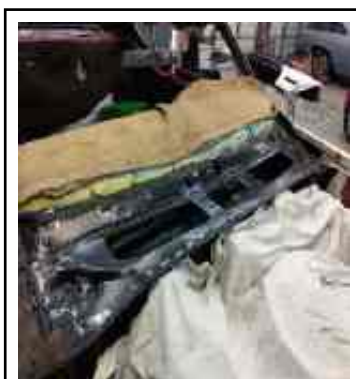
Cutlass "S" with the new cowlings sectioned into place
